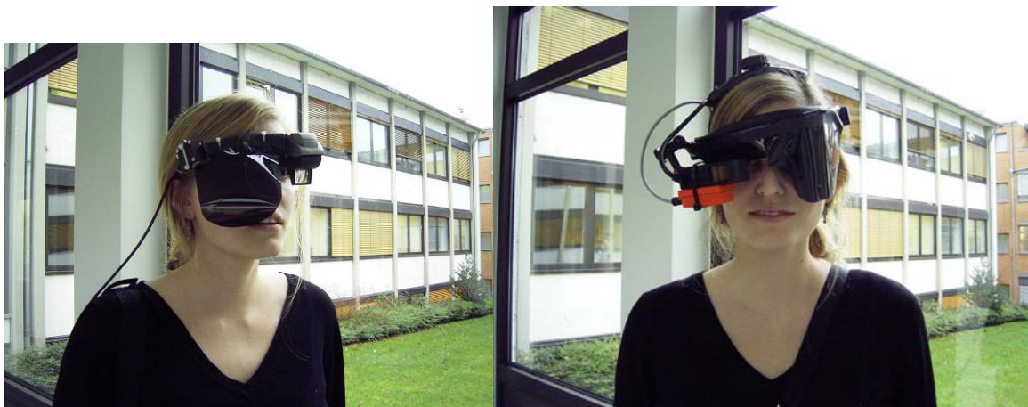
Figure 8 Close up at headsets, Shimadzu Data Glass 2 + IC3 (left), Liteye LE-750 +MTi (right)
